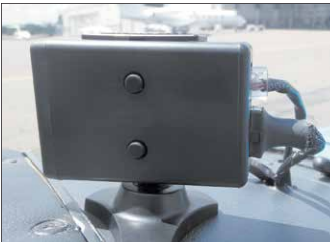
The SCc electro-mechanical lift transducer, top, is generally installed in the opposite wing of the stall warning vane. That's a rear view of the indexer/computer, with its interface cables.
