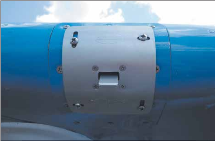
The SCc electro-mechanical lift transducer, top, is generally installed in the opposite wing of the stall warning vane. That's a rear view of the indexer/computer, with its interface cables.
