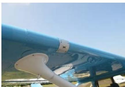
*Out on the wing, where angle of attack really counts, the SCx lift transducer measures angle of attack with great accuracy and responsiveness.*
