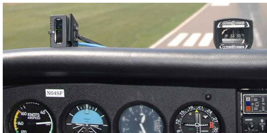
Safe Flight's new SCx angle of attack indicator. Photo courtesy of Safe Flight
